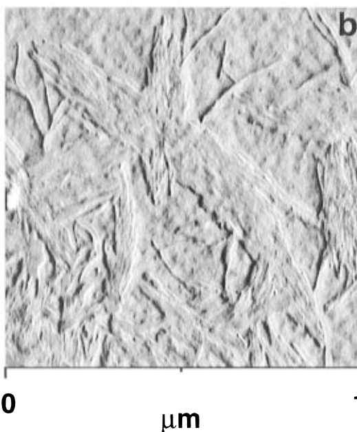
Figure 2. SFM micrographs of a thick film of polystyrene- block -PMPS with M_n = 18700 and 9000 and overall polydispersity M_w/M_n = 1.22 (a) before and (b) after degradation with 360 nm light.
